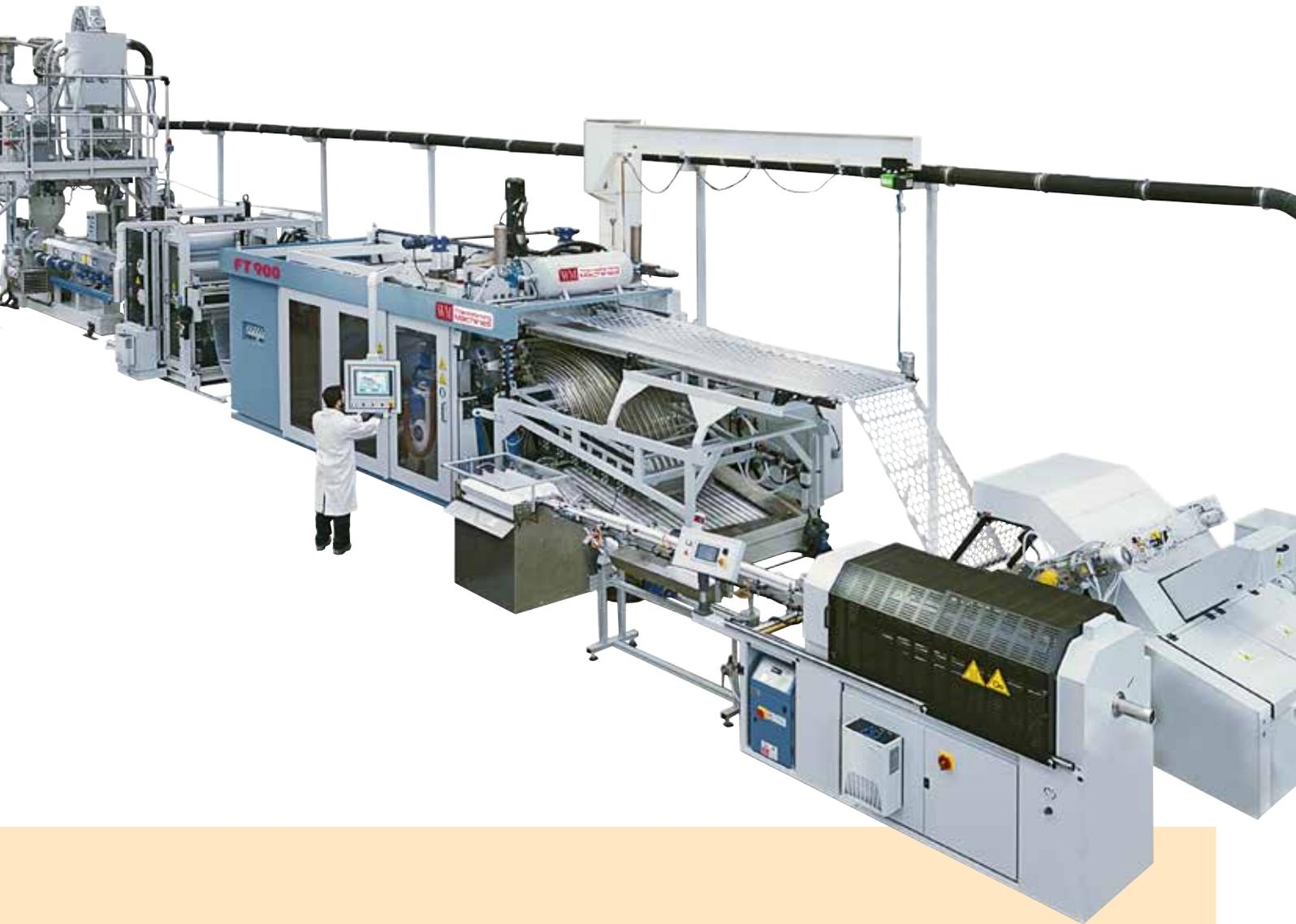
All FT machines can be supplied as an in-Line series, forming a real “production island” starting from the raw material up to the finished product, including the IN-LINE recycling of the granulated scrap.
