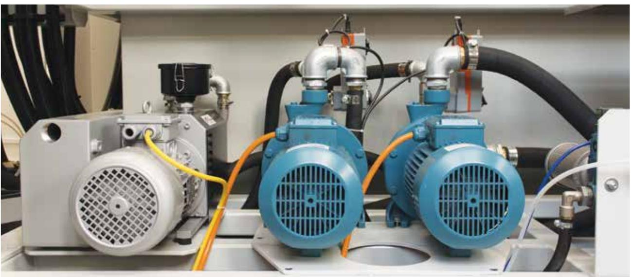
The TWIST 700 has integrated two independent mould temperature circuits to keep constant the  $\Delta T$  in  $2^{\circ}\text{C}$  between the upper and lower mould.
