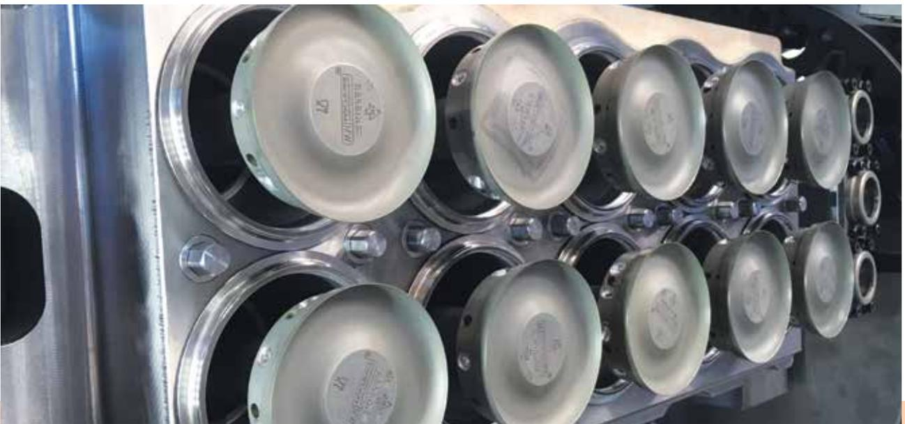
Electric extractor for better cycle synchronization is not requiring any mechanical stopper inside the mould, therefore reducing overall maintenance.
