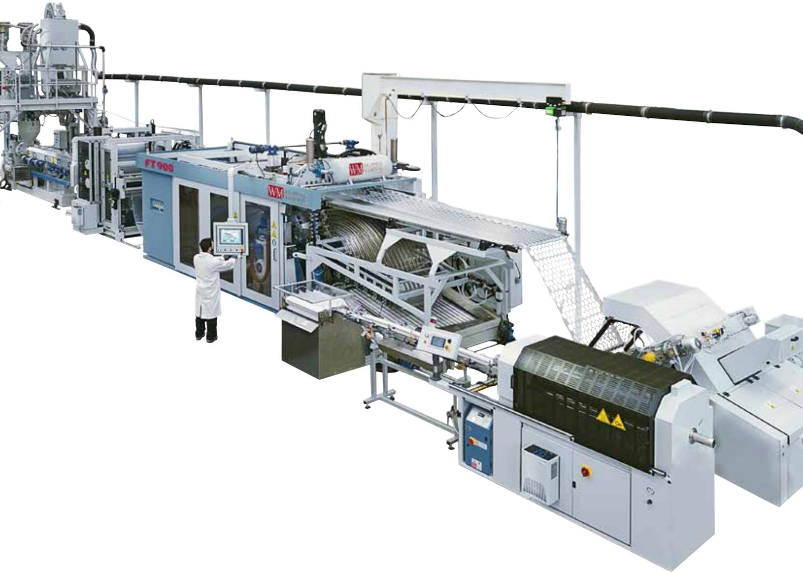
TWIST 700 machines can be supplied as an IN-LINE series, forming a real “production island” starting from the raw material up to the finished product, including the IN-LINE recycling of the granulated scrap.
