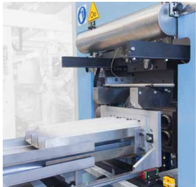
Thermoforming Machine TWIST 300 works with air pressure and simultaneous in-mould punching, vertical movement and 90° rotation of the lower platen.
